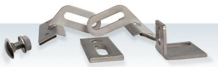
Manufactured from A2 stainless steel, the EJOT ATB-Plus is compatible with most common metal roofing materials. An integral EPDM adhesive rubber sealant on the base ensures quick weather-proof installation.
