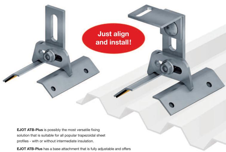
**EJOT ATB-Plus** has a base attachment that is fully adjustable and offers and multiple solar module options accommodating varying widths and heights. Installation is quick and clean - **ATB-Plus** comes with ready applied, self-adhesive EPDM sealant to ensure quick installation and a weather-proof fit.
