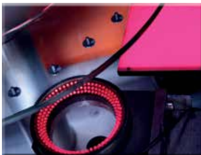
10 ppm sorted for 3 – 4 criteria, photo-optical
