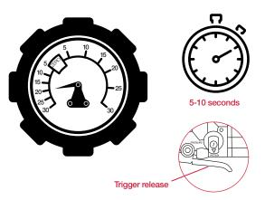
8 If the pressure does not hold steady and the needle drops, repeat the process, taking extra care to ensure the suction cup is firmly held over the fastener and washer. Increase the number of times you squeeze and release the pump handle.
