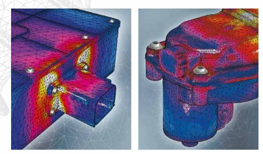
Stress analysis in the component under load
